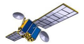
Some Cospas-Sarsat satellites only relay the distress message transmitted by the beacon. Other satellites relay the message and also gather details about the signal that will enable computers on the ground to estimate the beacon's location. Different kinds of satellites may be visible from your location at different times and, in remote areas, there can be an additional delay in the distress signal
